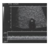
Registration indicates the position accuracy of the sample volume cursor of a Doppler image. The strongest and highest velocity signal is expected at the center of the vessel. When the sample volume position is inaccurate on Doppler images, the strongest signal is off-center.
