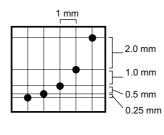
Axial resolution describes the scanner's ability to detect and dearly display dosely spaced objects that lie on the beam's axis. Using pin targets of decreased vertical spacing, the system's axial resolution is determined by locating the two resolvable pins with the smallest separation.
