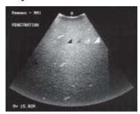
The point at which usable tissue information disappears or maximum depth of penetration is reached, can be defined simply as how far one can "see" into the phantom. Equipment sensitivity and noise determines the deepest echo signal which can be detected and dearly displayed.
