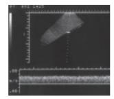
By forming Doppler signals into two different electrical channels, 90° out of phase, flow away from or toward the transducer is determined. Inadequate discrimination between channels appears as bi-directional even though flow is in one direction.
