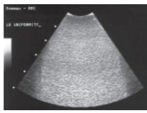
Ultrasound systems can produce various image artifacts and non-uniformities which in some cases mask variations in tissue texture. Common non-uniformities are horizontal bands in the image caused by inadequate handling of transitions between focal zones or vertical bands indicating inactive or damaged transducer elements.
